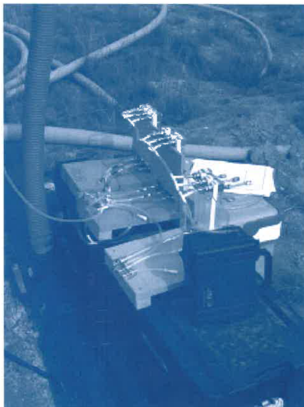
Figure 5.3 | Sampling tubes and rotameter assemblies
