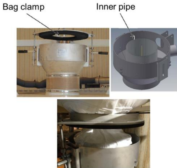
Figure 12: Activated carbon 'dust free' metering system
